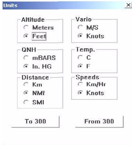
Select from this screen the desired units of measurement for Altitude, Distance, and Speeds to be reported on the flight record. Click on "To 300" to send these choices to the 302A/CFR or "From 300" to obtain the current settings from the instrument.
