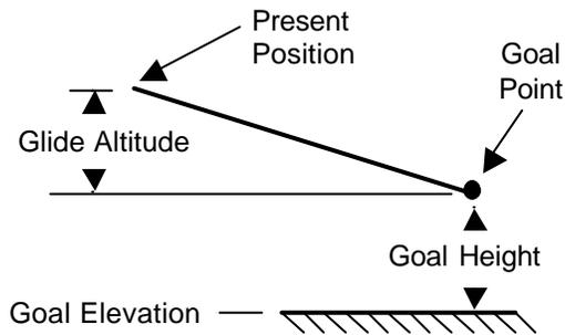
$$\text{Diff.} = \text{Altimeter} - \text{Glide Altitude} - \text{Goal Height} - \text{Goal Elevation}$$
