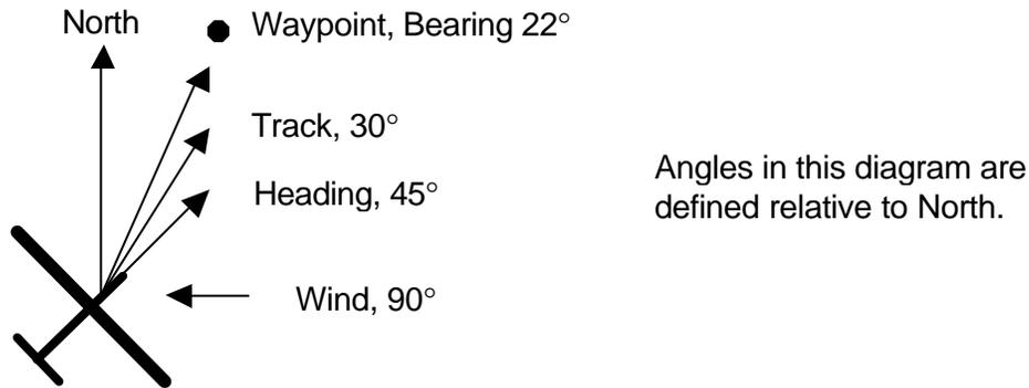
Bearing is the angle of the line between the glider's position and the Waypoint.
